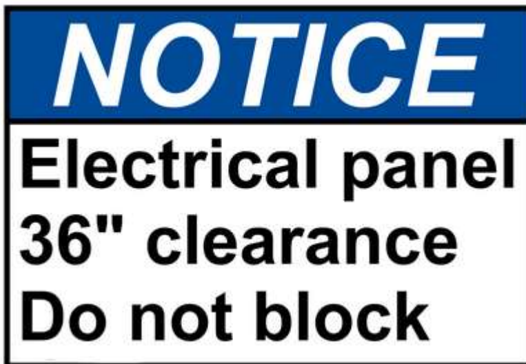
Figure 23. Electrical panel clearance label.
