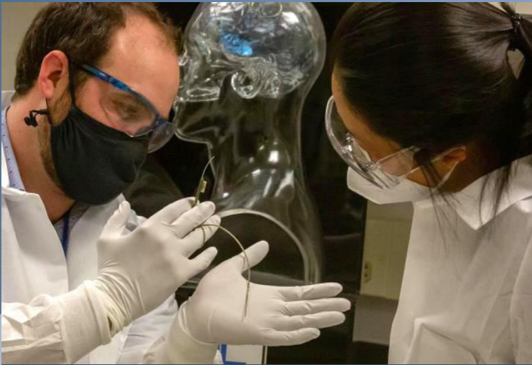
In a study at the University of California, San Francisco, neurologists place thin-film multi-electrode arrays developed at Lawrence Livermore on the exposed hippocampus of patients undergoing epilepsy-related surgeries. Pictured are LLNL researchers Michael Triplett (left) and Jenny Zhou.
