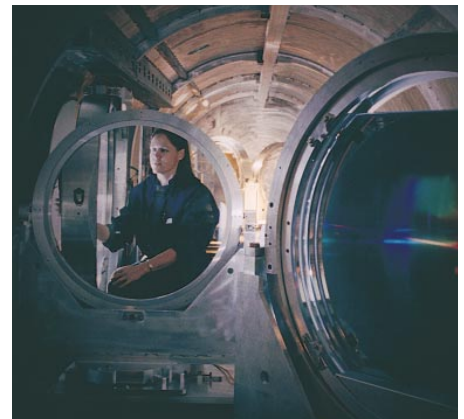
The chirped-pulse amplification technique makes it possible for the Petawatt laser's high-power pulses to pass through laser optics without damaging them. Before amplification, low-energy laser pulses are passed through diffraction gratings to stretch their duration by as much as 25,000 times. After amplification, the pulses are recompressed back to near their original duration. Because the pulses pass through the laser optics when they are long, they cause no damage.
