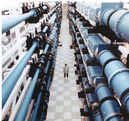
The chirped-pulse amplification technique makes it possible for the Petawatt laser's high-power pulses to pass through laser optics without damaging them. Before amplification, low-energy laser pulses are passed through diffraction gratings to stretch their duration by as much as 25,000 times. After amplification, the pulses are recompressed back to near their original duration. Because the pulses pass through the laser optics when they are long, they cause no damage.
