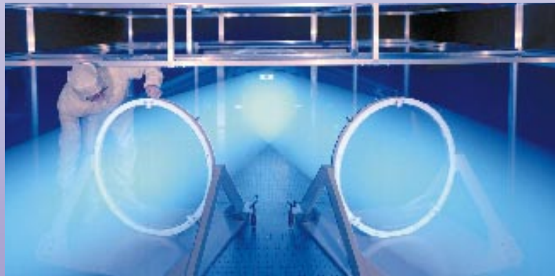
In this booth, interference lithography exposes a layer of photoresist in a groove pattern.
