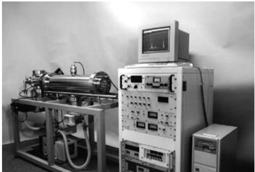
Figure 3. Our laboratory-size ion-storage trap/time-of-flight (IT/TOF) instrument. We are currently designing a smaller portable instrument.
