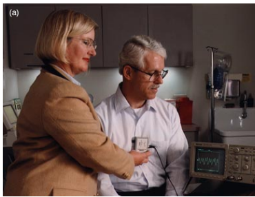
Figure 10. (a) An MIR cardiac monitor. (b) Its output (upper trace) is distinctly different from that obtained by a conventional EKG (lower trace). We are working with physicians to correlate the radar signals with physiological functions.
