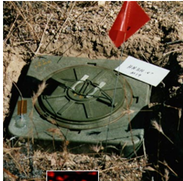
Figure 8. A typical plastic antitank mine is shown (top) before burial at the Nevada Test Site. MIR technology was used (bottom) to image the mine at three depths, or horizontal "slices."
