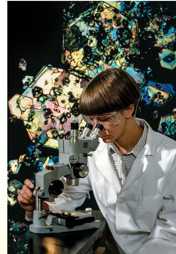
Crystals of TATB (triamino-trinitrobenzene), which are shown magnified in the background, are examined under a microscope.
