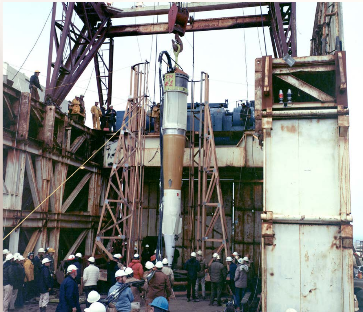
A Spartan missile body with the nuclear device is lowered downhole for the Cannikin event. The test was successfully conducted on November 6, 1971, on Amchitka Island, Alaska.
