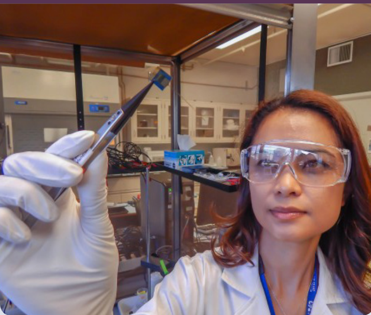
Lawrence Livermore engineer Vanessa Tolosa holds up a flexible electrode array that gets implanted into animals to record brain signals, as part of a project that may help restore memory.
