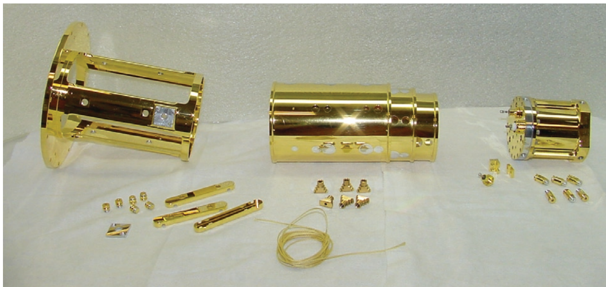
All parts of the germanium detector assembly (right), its thermal shielding (center), and its external cage (left) are highly polished and gold-plated to minimize radiative-heat transfer.
